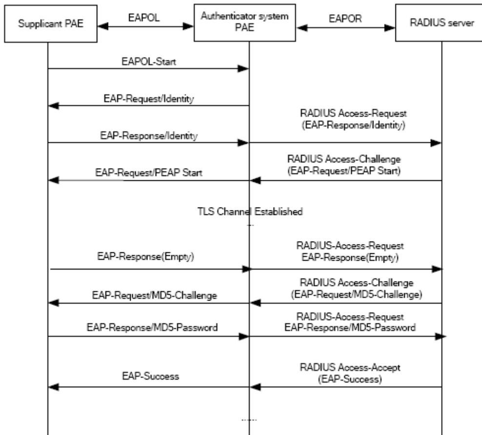
**Figure 42-11:** the Authentication Flow of 802.1x PEAP
