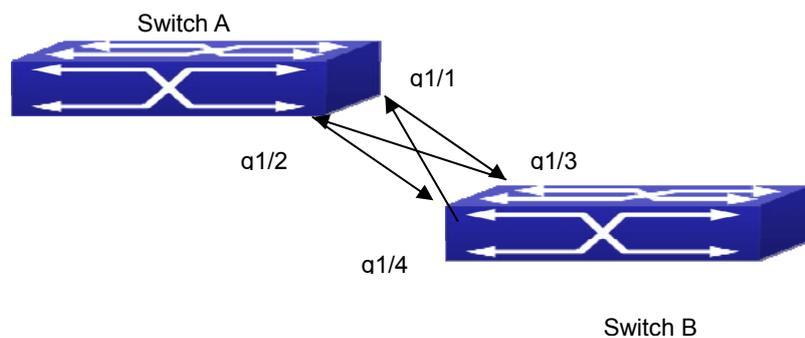
Figure 10-1: Fiber Cross Connection
