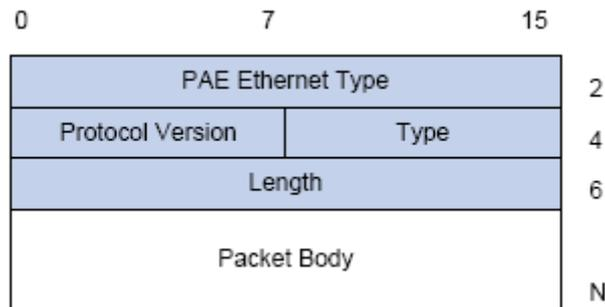
**Figure 42-3:** the Format of EAPOL Data Packet
