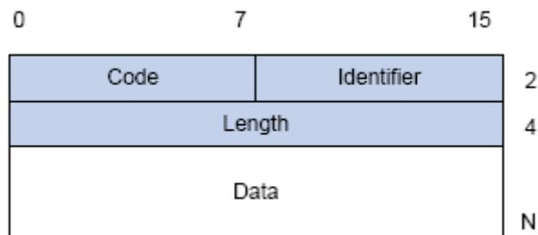
**Figure 42-4:** the Format of EAP Data Packets
