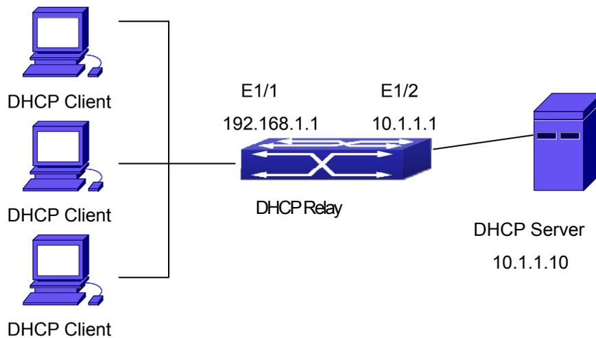
**Figure 31-3:** DHCP Relay Configuration
