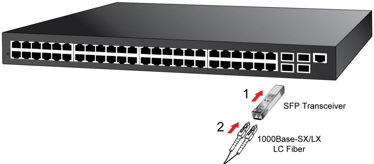
**Figure 2-7** Plug in the SFP transceiver
