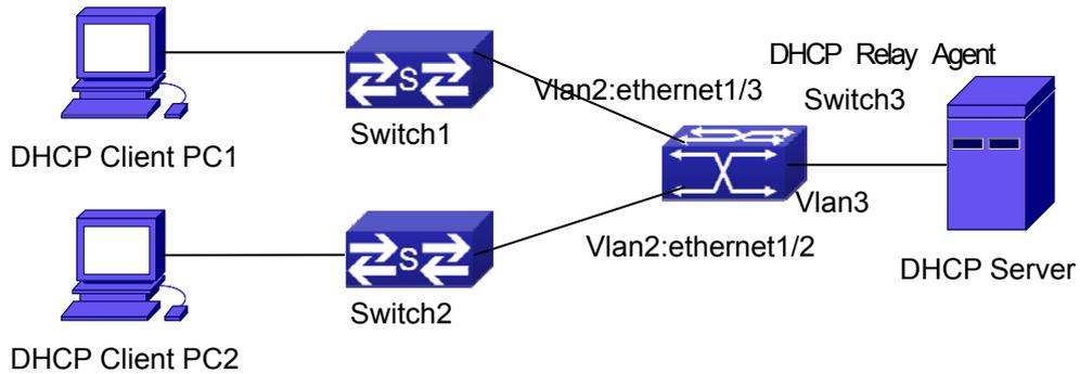
**Figure 33-1:** A DHCP option 82 typical application example
