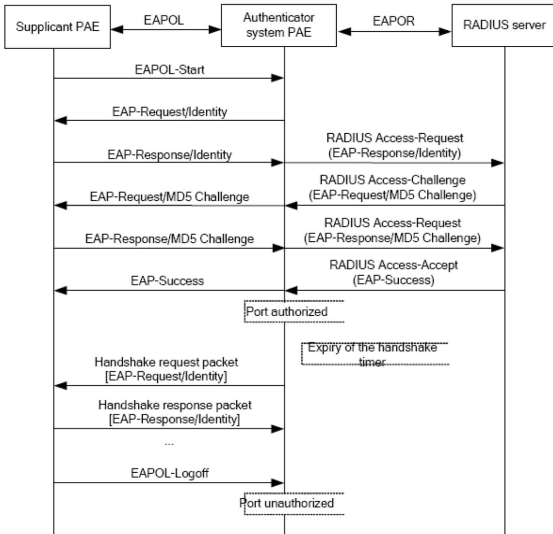
**Figure 42-9:** the Authentication Flow of 802.1x EAP-MD5
