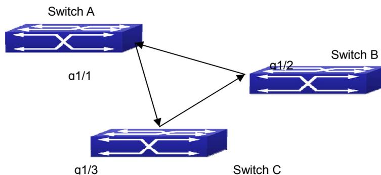
Figure 10-2: One End of Each Fiber Not Connected
