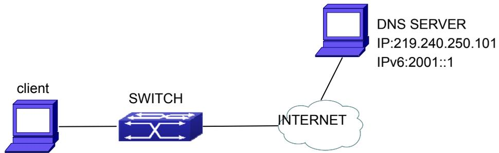
**Figure 65-2:** DNS SERVER typical environment
