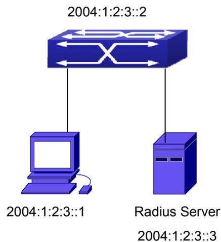
**Figure 47-3:** The Topology of IPv6 Radius configuration
