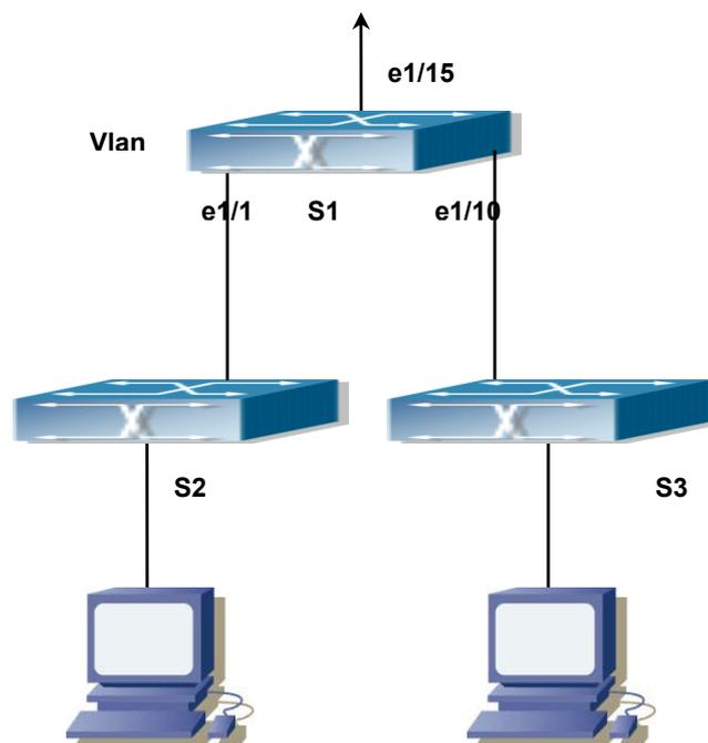
**Figure 8-1:** Typical example of port isolation function
