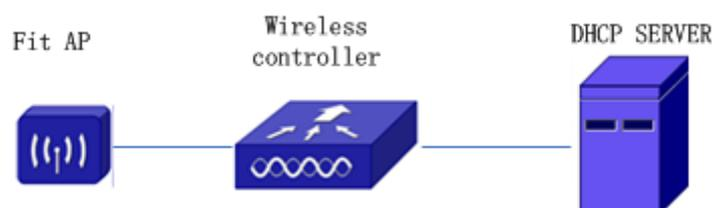
**Figure 34-1:** Typical DHCP option 60 and option 43 topology
