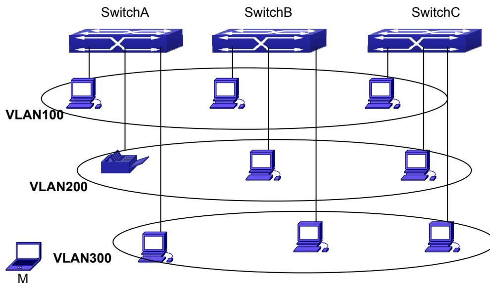
Figure 20-8: Typical topology application of dynamic VLAN
