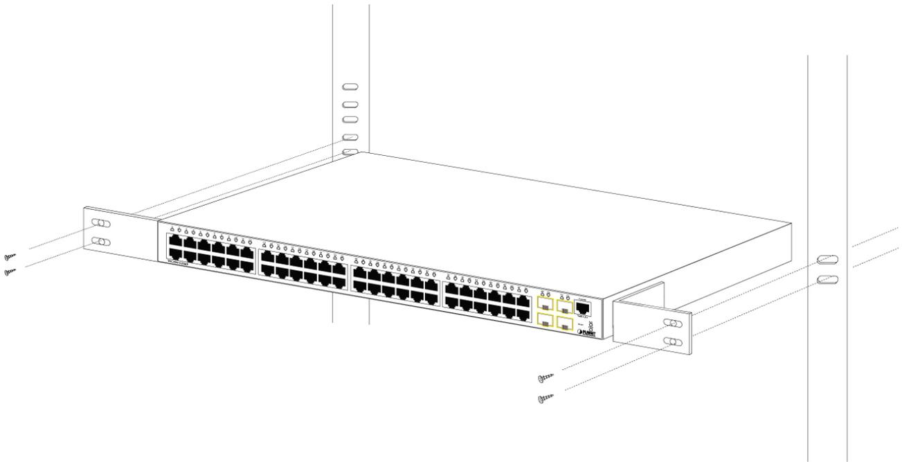
**Figure 2-6** Mounting WGSW-52040 in a Rack
