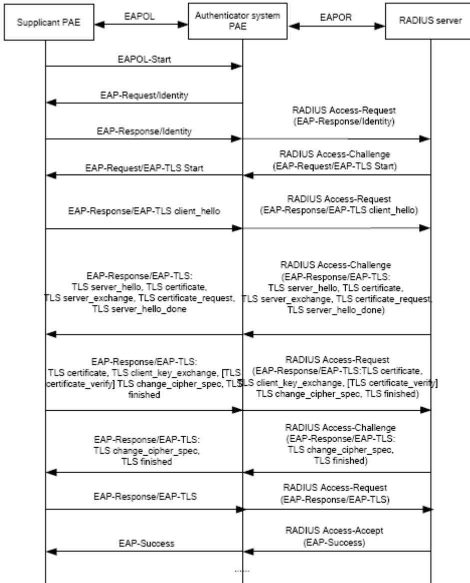
Figure 42-10: the Authentication Flow of 802.1x EAP-TLS
