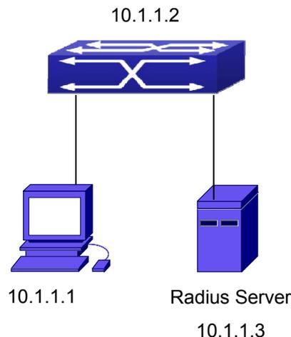
**Figure 47-2:** The Topology of IEEE802.1x configuration
