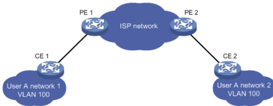
Figure 18-1: BPDU Tunnel application
