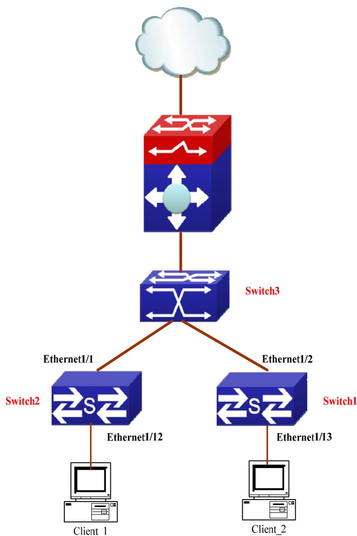
Client\_1 and Client\_2 means two different user's PC installed IPv6 protocol, respectively connect with port Ethernet1/12 of Switch1 and port Ethernet1/13 of Switch2, and enable the source address check function of SAVI. Ethernet1/1 and Ethernet1/2 are uplink ports of Switch1 and Switch2 respectively, enable DHCP trust and ND trust functions. Aggregation Switch3 enables DHCPv6 server function and route advertisement function.
