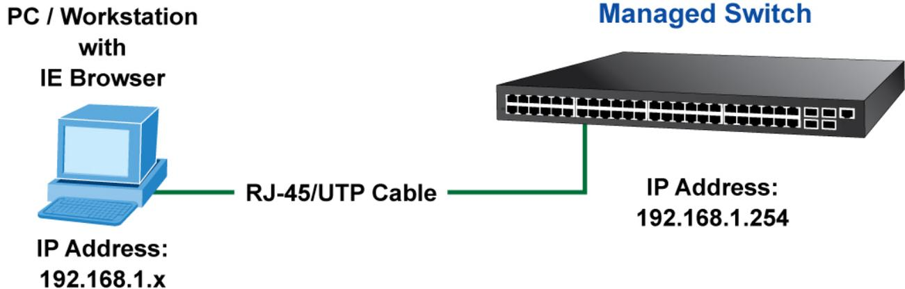
**Figure 3-6** Manage the switch by Telnet
