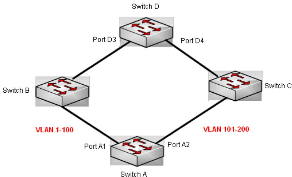
**Figure 56-2:** VLAN load balance
