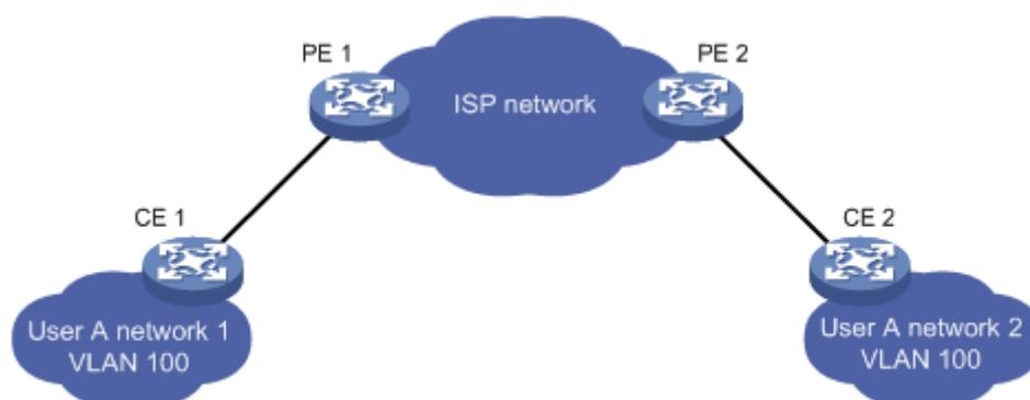
**Figure 18-2:** BPDU Tunnel application environment
