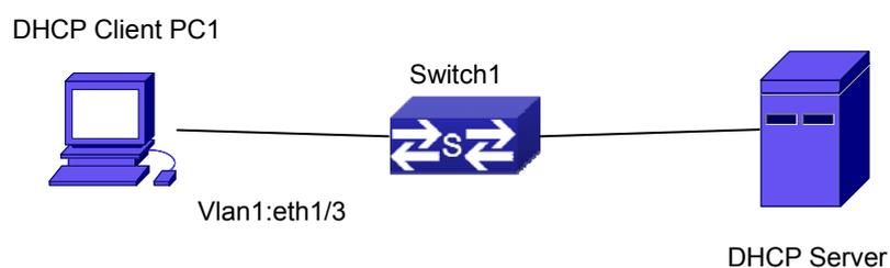
**Figure 37-1:** DHCP option 82 typical application example
