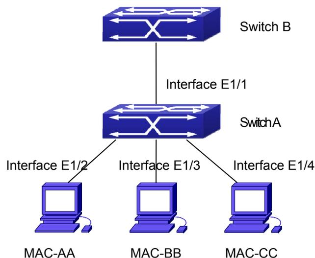
**Figure 35-1:** DHCPv6 Snooping option schematic
