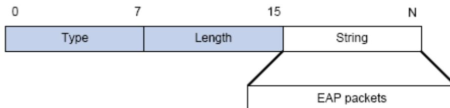
Figure 42-6: the Encapsulation of EAP-Message Attribute
