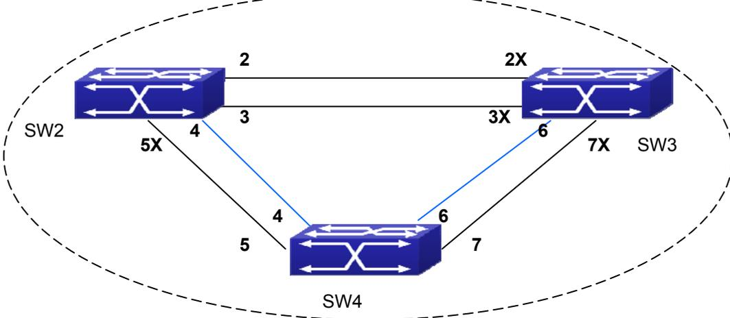
**Figure 22-5:** The Topology Of the Instance 4 after the MSTP Calculation
