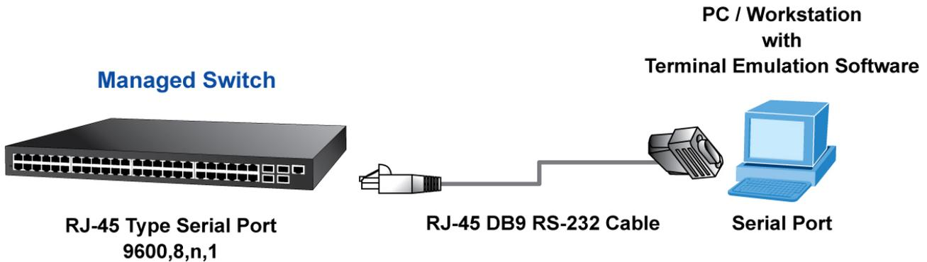
Figure 3-1 Out-of-band Management Configuration Environment
