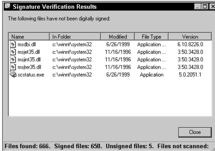
FIGURE 5-57 Unsigned files detected by sigverif.exe
