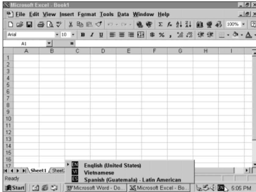
FIGURE 5-46 Selecting an input locale for an application
