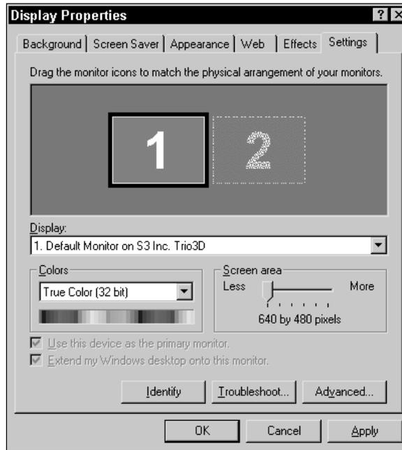
FIGURE 5-19 Configuring multiple-display support
