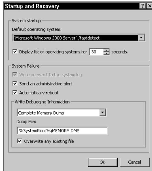
FIGURE 5-70 Configuring startup and recovery options
