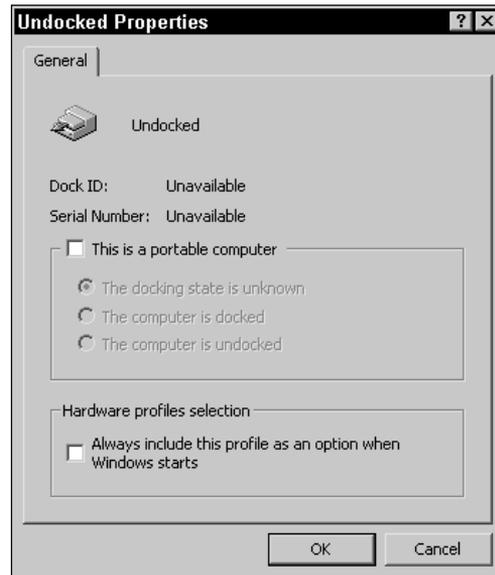
FIGURE 5-65 Configuring a new hardware profile
