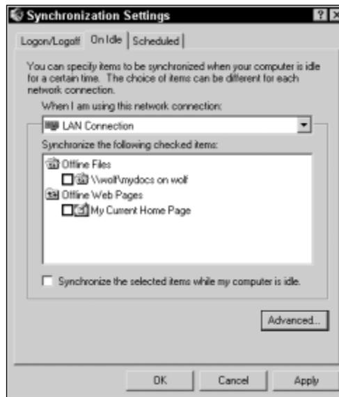
FIGURE 5-28 Configuring idle settings for offline files
