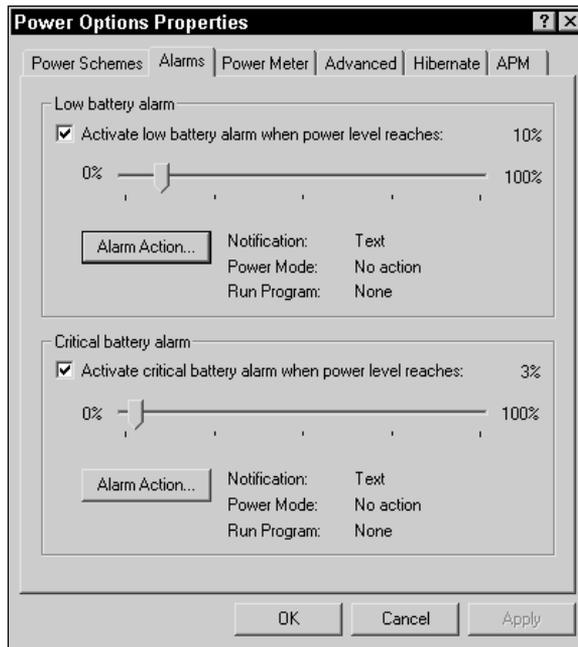
FIGURE 5-39 Configuring battery alarms
