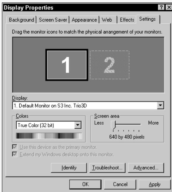
FIGURE 5-77 Configuring multiple display support
