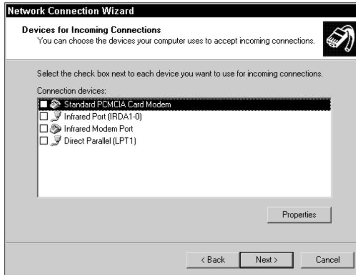
FIGURE 15-4 Selecting connection devices
